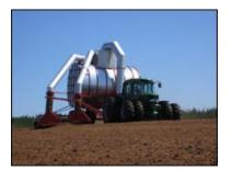
Figure 1d – Collecting the dry surface peat layer with a vacuum harvester
