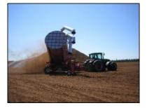
Figure 1e – Dumping the collected peat at the end of the production fields
